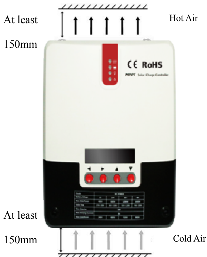
Figure 2.1 Installation and Heat Dissipation
