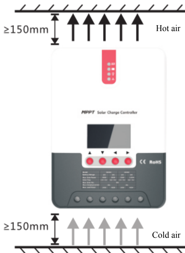
Fig. 2.1 Installation and heat dissipation
