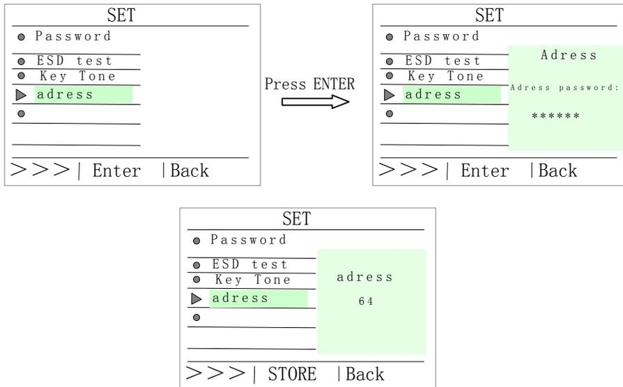
2. After setting, press “STORE” save, and press “Back” key return parameter setting interface, and press “Back” key return main menu.
