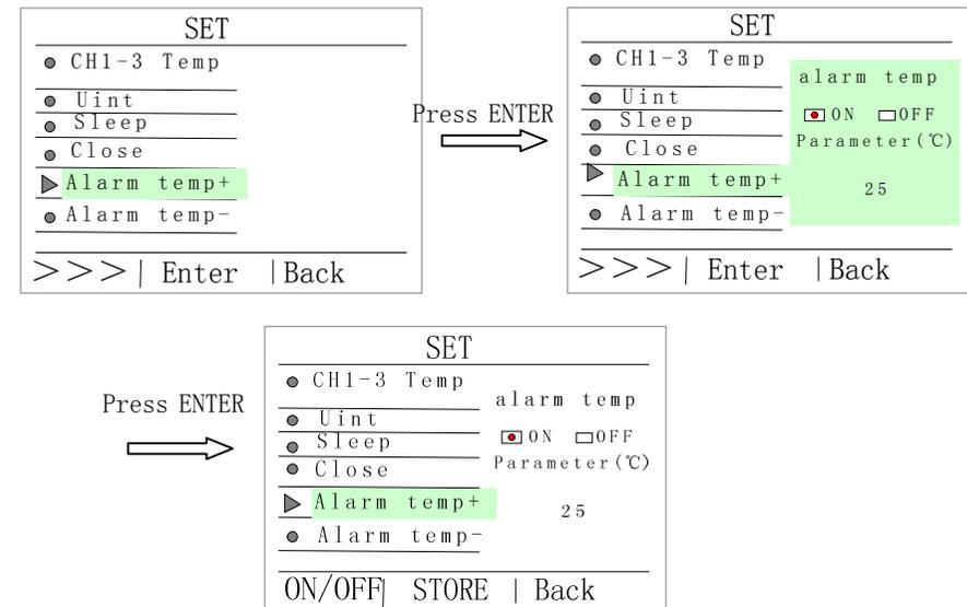
2. after setting alarm temperature+, press “store” affirm, press “Back” return parameter setting interface, press “Back” again, return menu interface.
