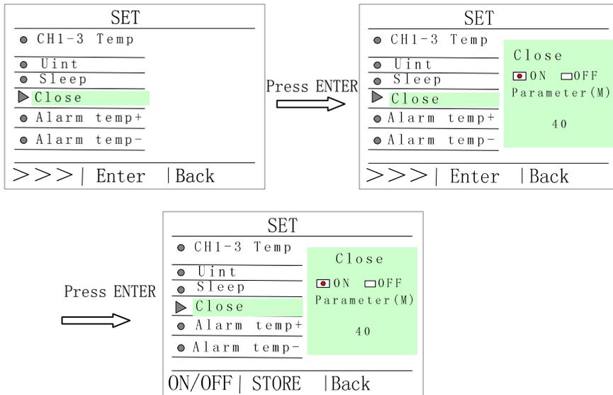
2. After setting close time ,press “STORE” key affirm, press “Back” key return parameter setting interface, press “Back” again, return setting interface.
