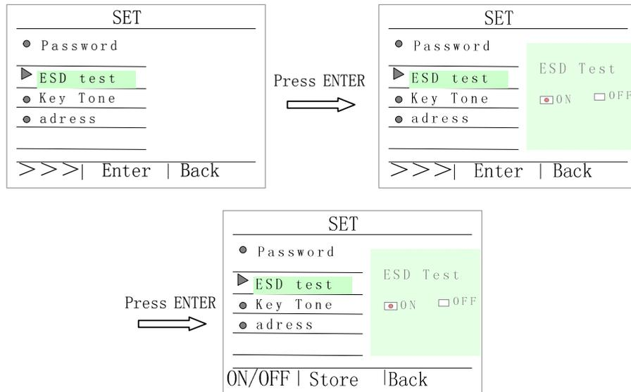
△ **Note: when select ON, the ground hole must be connect with ESD ground, otherwise, alarm hint (ESD in main interface show as red)**
