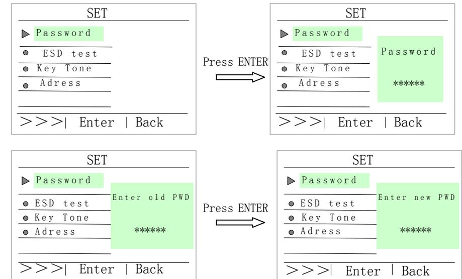
△ Note: after change password, the temperature cannot be modify, enter into parameter setting interface with new right password.
