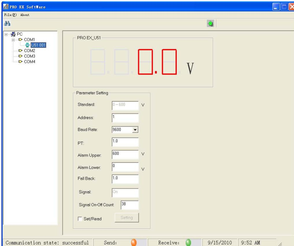
In the parameters setup box, the user can setup the parameters as PT, CT, upper limit, lower limit, and fall back value. Click “setup” (First, please choose “Set/Read”) after fill in the value and the following Fig appears:
