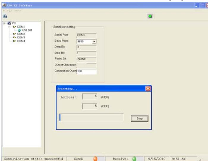
**Note:** When meters connect with com. at the same time, please make sure all the meters addresses are different, if not, please setup different address in the firmware, after that, It can be searched from the known smallest address. Click “stop” for stopping searching when it searching over the biggest address,
