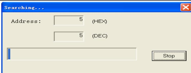
The user can choose the number without address for start to searching the corresponding firmware meter which had been set. 5 can be chosen as start address if the known smallest number for firmware address as 5, and the software will search meters between 5 and 255. The progress as following:
