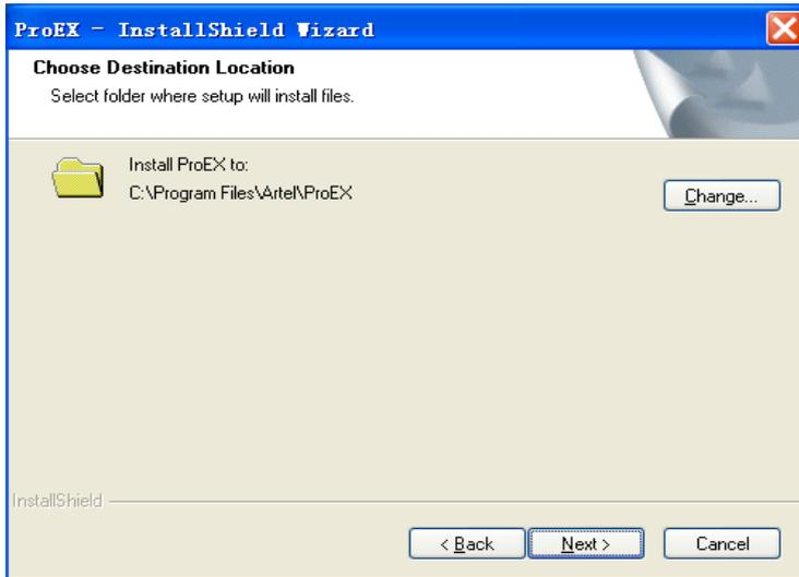
3) Change the installation file by clicking “Change”, if not, the progress is installed in the file C as \ProgramFiles\Artel\ProEX automatically. Click “Next” to enter the next page;
