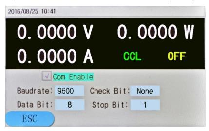
**Step 3:** Select the **Baud Rate** menu item via and keys, set the parameter to 9600 via the knob and then press the key to enter;
