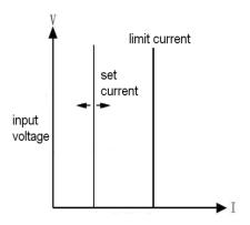
Fig. 2-13 Current Limit Function in CV Mode
