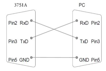
**RS232** interface is the standard configuration of the load. Correctly connect the load and the PC via the RS232 interface shipped with the load. Select RS232 interface in the MENU, and set the Baud rate, parity, data bit, stop bit and so on corresponding parameters. Set the same parameters in the PC software. Then input the SCPI commands in the PC software interface to operate the load.
