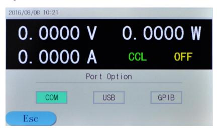
**Step 2:** Select the **GPIB** menu item via and keys, then press the key to enter;
