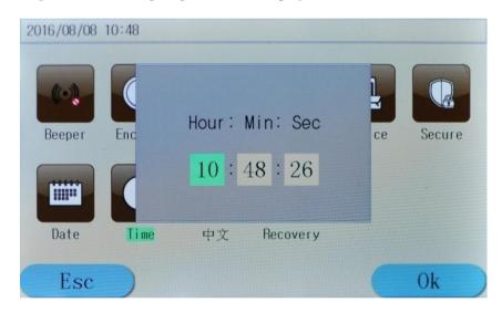
Step 4: Select Hour, Min and Sec via , keys and regulate the level via the number keypad or the knob. After pressing key, the initial interface will display the set time;
