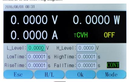
Step 2: Select "L\_Level" via key or and keys; enter the transient low level 10 by the number keypad, or via knob with and keys; then press key to confirm:
