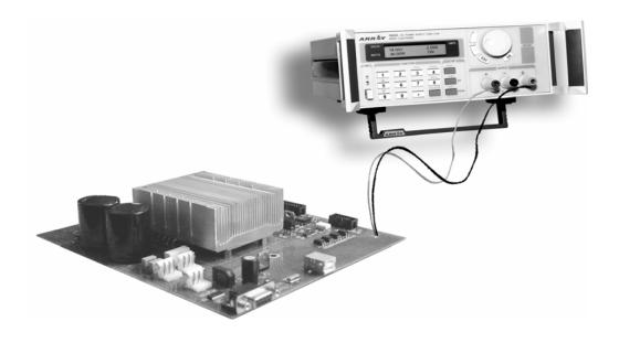
Fig. 2-1 Connect the Power Supply to the load
