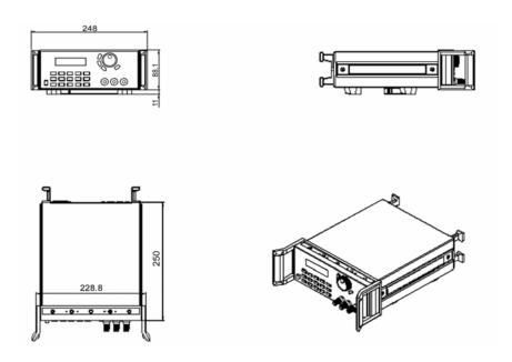
Fig. 1-1 Dimensions of 364X Series Programmable DC Power Supply
