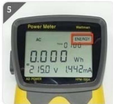
"Energy" sign is displayed at the above right of LCD screen and start integration.
