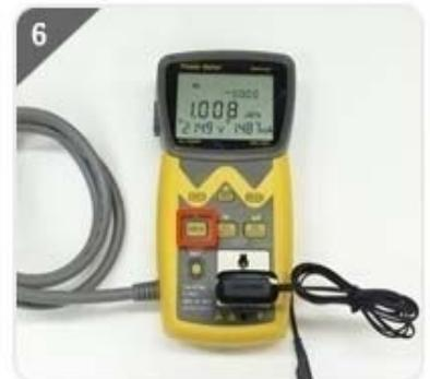
After wattage integration press DISPLAY button and change to CO<sub>2</sub> emission mode.
