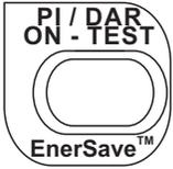
When Depressing the "ON-TEST" Button, the instrument starts up or resets.
