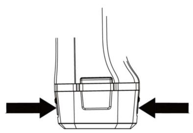
Figure 2-1 Remove Battery Base
