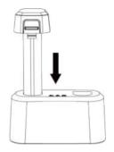
Figure 2-2 Charge Battery
