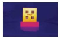
7. Adjust the target's optical image with navigation buttons until it overlaps with the thermal image, and press ⊚ k. The well-overlapped image is shown as follows.
