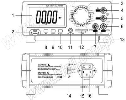
1. LCD2. Power switch3. Function knob4. VΩHz input terminal5. COM6. Less than 2A current input terminal7. 20A current input terminal8. Backlightswitch9. Hold switch10. AC+DC measuring switch11. hFEplug12. Capacitancemeasuring plug13. Bracket14. 110V/220V transfer switch15. fuse16. Power plug
