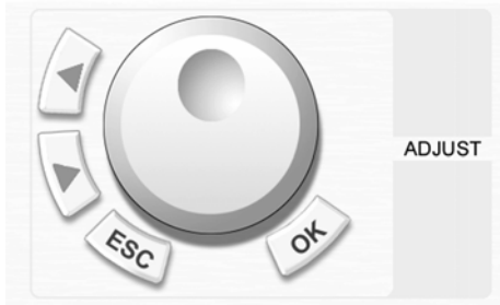
Fig.1-5 Rotary knob and function keys
