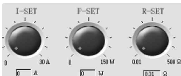
Fig.2-7 Current, Power, Resistance setting dial
