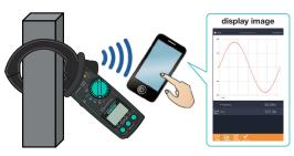
Download and install our special application "KEW Power \*" in your smartphone or tablet device for logging the measured values. Remote monitoring of voltage, current, power, trend graph of harmonics, and wave form is possible with "KEW Power \*"; this is helpful for simple Power Quality check. Measured values can be saved in your smartphone or tablet device in csv format: the data is editable in excel format.
