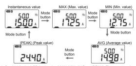
Range is fixed while the LCD is showing MAX, MIN, AVG, or |PEAK|. The auto-ranging function is reactivated when switching the display to instantaneous value.
