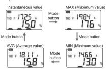
Range is fixed while the LCD is showing MAX, MIN, or AVG. The auto-ranging function is reactivated when switching the display to instantaneous value.
