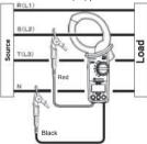
Another press of item switching button  $[\blacktriangleright]$  changes measurement object from S(L2) to T(L3).
