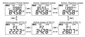
A long press of mode button clears measured results and the screen returns to the initial measurement setting screen.
