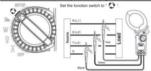
According to the wiring system of Three-phase 3-wire and Three-phase 4-wire to be tested, the results are displayed as the following table shows. Each number represents the connected phase order.
