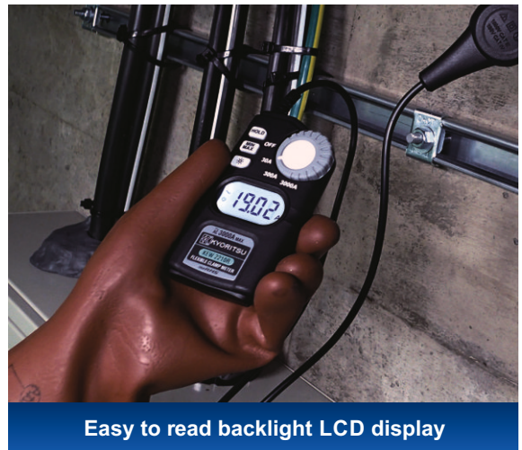
Easy to clamp a wire in hard-to-reach narrow spaces
