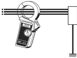
3-phase 3-wire system. (in 4-wire system with neutral clamp onto all 4 wire)
