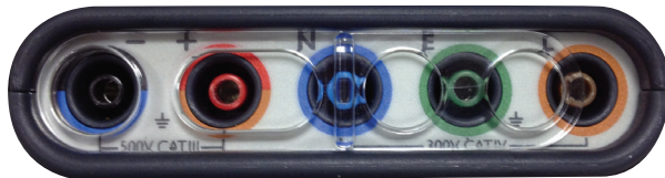
Fig.1 Interlock in position for Continuity and Insulation testing
