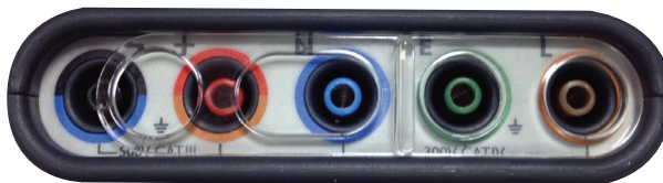
Fig.2 Interlock in position for RCD & Loop testing
