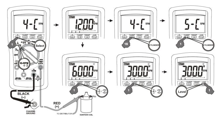
Press (4.2) button momentarily to select through **RPM** $(\frac{2}{4})$  for 4-stroke, **RPM**(2) for 2-stroke and DIS, and **RPM**(2) **M** for special 2-stroke waste ignition engine
