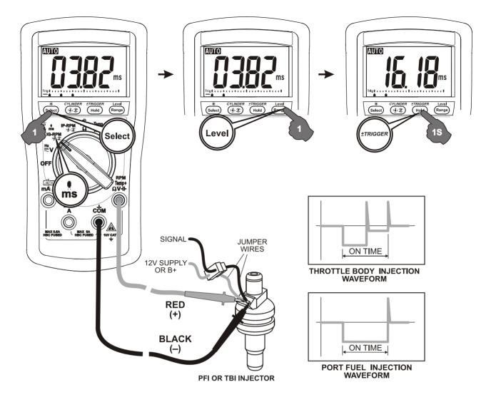
Trigger level defaults at 3. Press the Level (RANGE) button momentarily to select another trigger level. If the reading becomes unstable, select lower sensitivity to avoid electrical noise. If the reading shows zero, select higher sensitivity. Number of Bar-graph pointer is used to indicate sensitivity selected.
