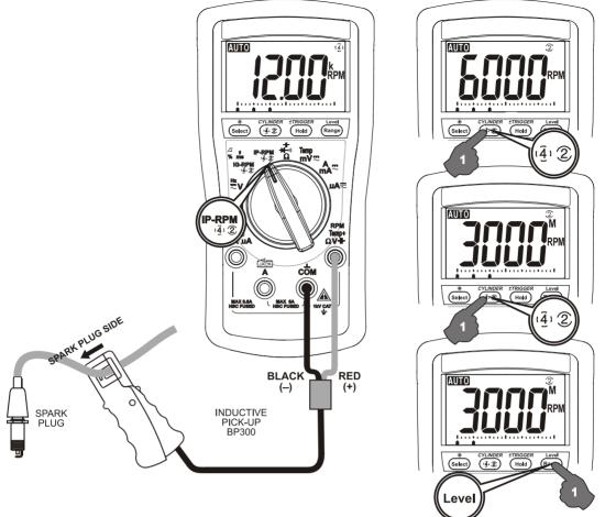
Press (4,2) button momentarily to select through **RPM**<sup>4</sup> for 4-stroke, **RPM**<sup>2</sup> for 2-stroke and DIS, and **RPM**<sup>2</sup> **M** for special 2-stroke waste ignition engine
