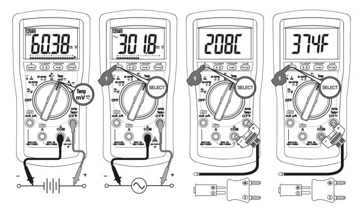
Note: Be sure to insert the banana plug K-type temperature bead probe Bkp60 with correct **+** – polarities. You can also use a plug adapter Bkb32 (Optional purchase) with banana pins to K-type socket to adapt other standard K type mini plug temperature probes.
